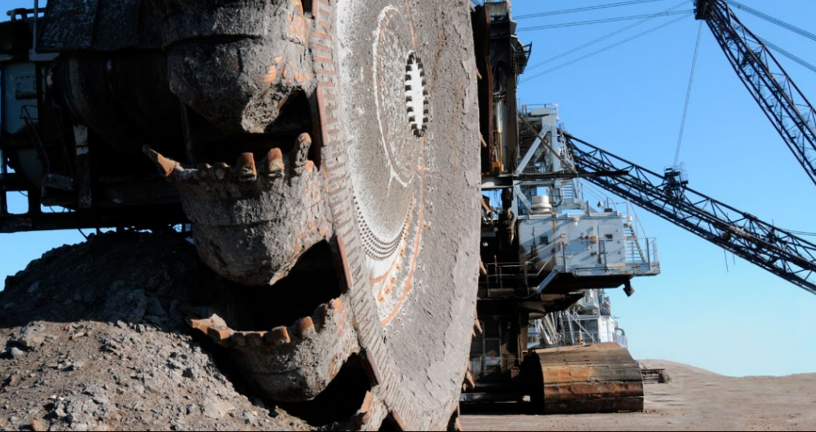
Bucketwheel reclaimer at an oil sands mine in Alberta, Canada
