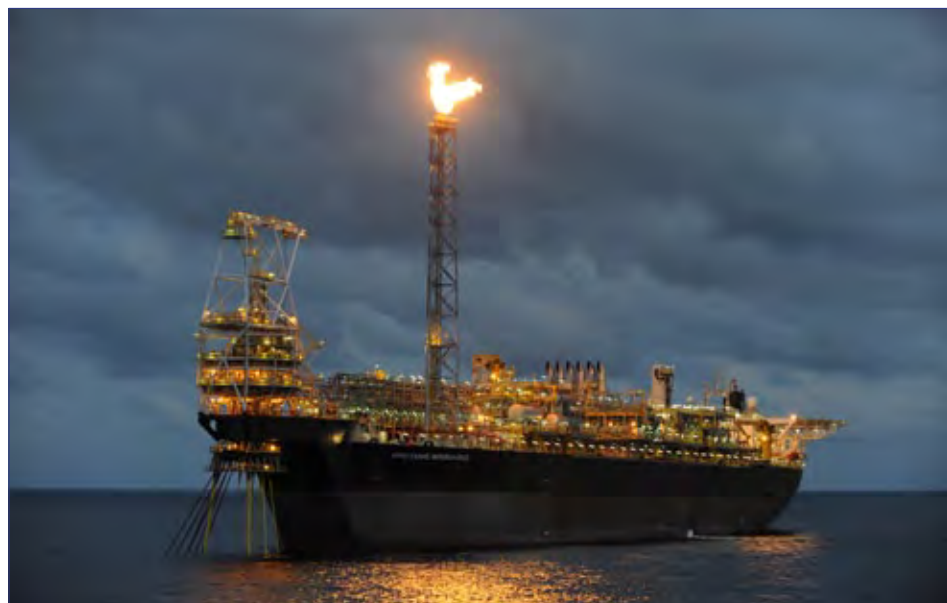
Anadarko's floating, production and storage (FPSO) vessel in Ghana's Jubilee offshore field
