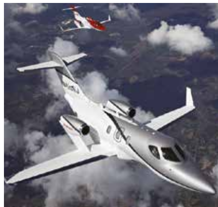
HondaJet's Over-The-Wing Engine Mount cuts drag; ups performance
